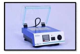
Rivotek Dry Bath dual block non porous aluminium blocks, along with a competitive range of interchangeable blocks. It is designed for a variety of applications, including restriction digest, denaturing DNA, BUN, melting agar, coagulation studies, hybridization and Hot Start thermo-cycled reaction.
