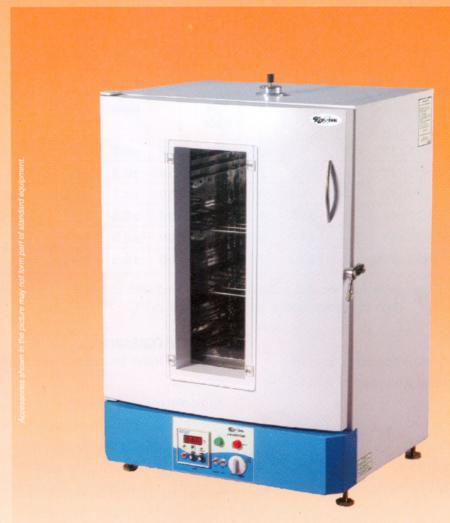
Current models of Bacteriological Incubators are manufactured with full inside transparent acrylic door & outside full MS door instead of single outside door with glass window. Controller design is also improved.
